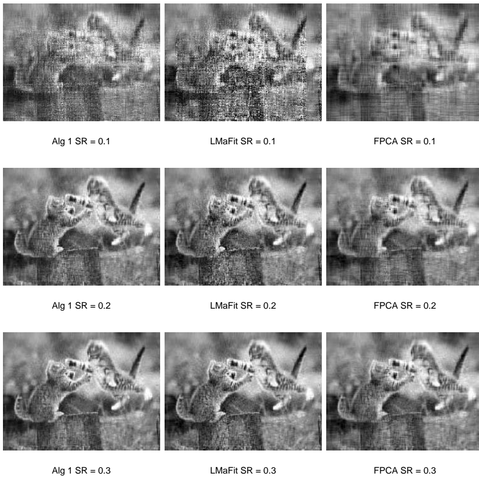
Figure 5: Recovered 768 \times 1024 Kittens with estimate rank q = 40 by Algorithm 1 (left), LMaFit (middle), and FPCA (right)
