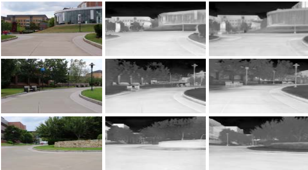
Figure 7: Image samples translated from color visible domain to infrared radiation domain on our collected dataset. The first column: color image input. The second column: translated thermal image output.
