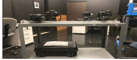
Figure 2: Our camera system, which involves a thermal camera (the most left one) and two SLR cameras (second left one and the most right one). The most right thermal camera is to pair up with the other thermal camera to generate ground truth depth map, which is not used in training process.
