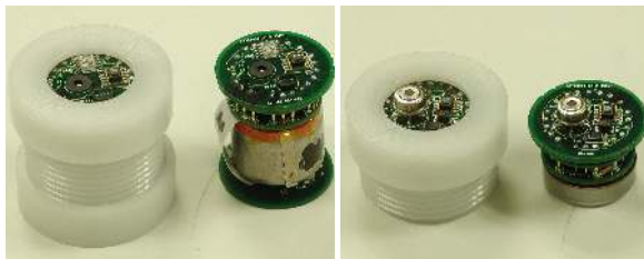
Figure 3: Mote configurations used in the deployment: weather mote (left) and burrow mote (right)
