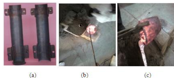
Figure 2. (a) Permanent mould for 40 mm diameter round bar (b) Mixing again manually before Pouring (c) Pouring mixture of molten Al and SiC particles
