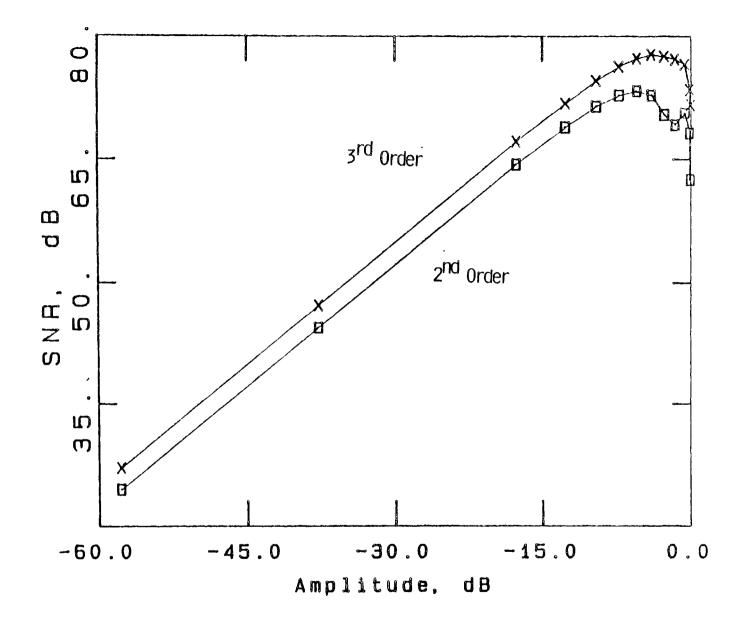
Fig. 16. Calculated SNR for 2<sup>nd</sup> and 3<sup>rd</sup> Order Modulator,  $\frac{f_s}{f_b} = 256$
