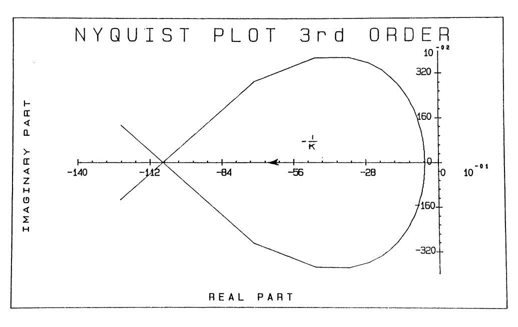
Fig. 23 Nyquist Plot 3<sup>rd</sup> Order Modulator ( $\alpha_1 = 0.1$ ,  $\alpha_2 = 0.1$ ,  $\alpha_3 = 1.0$ )
