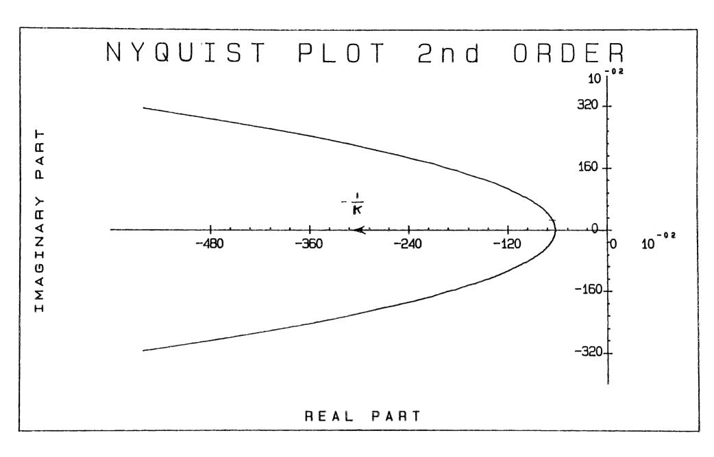
Fig. 22 Nyquist Plot 2<sup>nd</sup> Order Modulator ( $\alpha_1 = 0.5$ ,  $\alpha_2 = 1.0$ )
