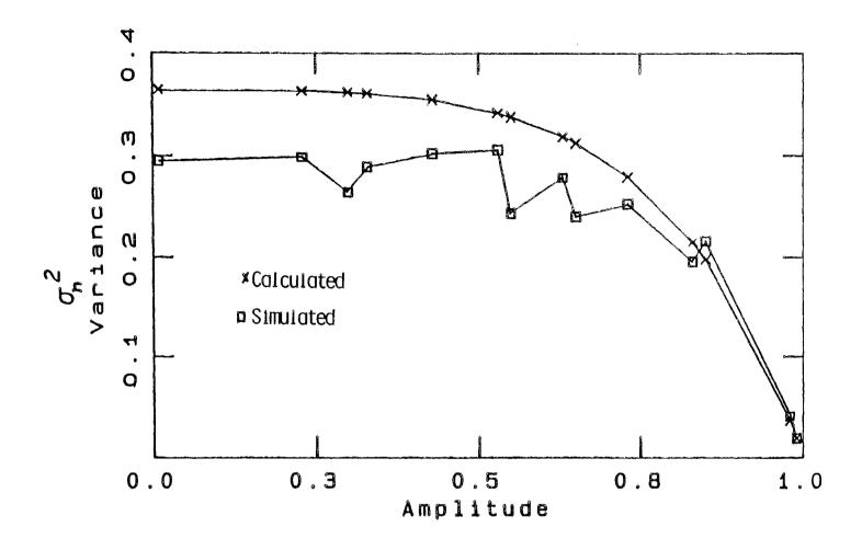
Fig. 10. Calculated and Simulated Additive Noise Variance  $\sigma_{n}^{\,2}$
