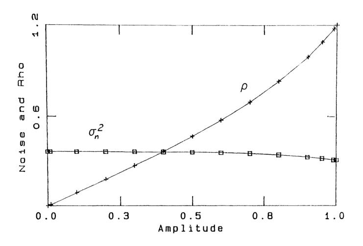
Fig. 11. Calculated Additive Noise Variance,  $\sigma_n^2$ , and  $\rho$  Sinusoidal Input
