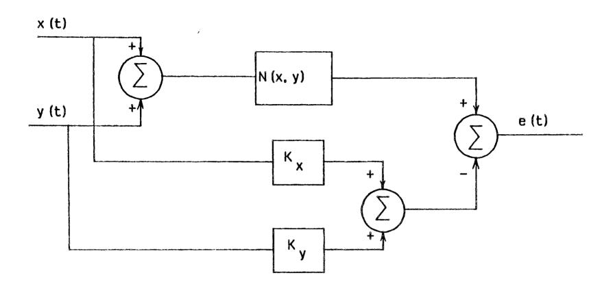
Fig. 6. Minimum Mean Square Error Linearized Gain Modeling of Nonlinearity
