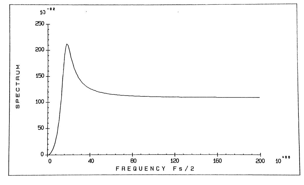
Fig. 13. Calculated Noise Spectrum,  $K_n = 0.1$
