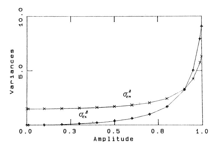
Fig. 21. Calculated Variances at Quantizer Input, 2<sup>nd</sup> Order Sinusoidal Input
