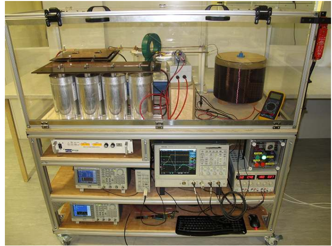
Fig. 3. The clamped inductive measurement test rig, consisting of a series of bank capacitors, inductors and copper plates to minimize the effect of parasitic inductances.
