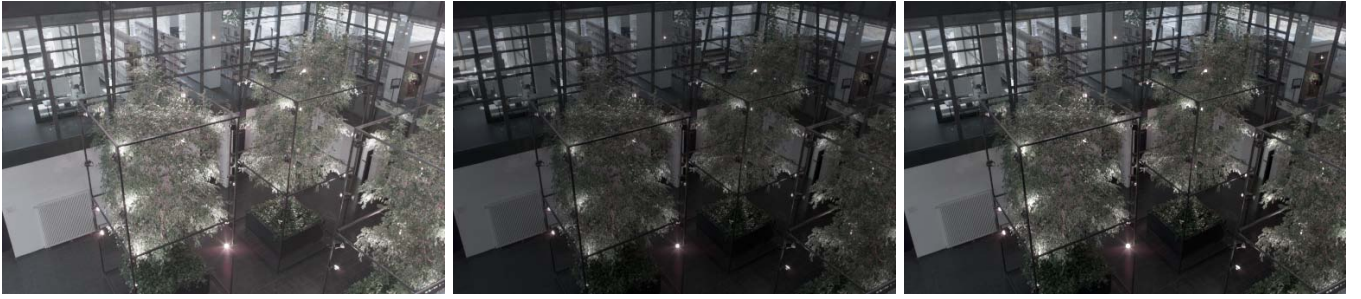
Figure 3. Left: TM output using the Naka-Rushton equation. Middle: TM output using a logarithmic mapping (Weber-Fechner’s law.) Right: TM output of the first stage of our method, eq. (6).
