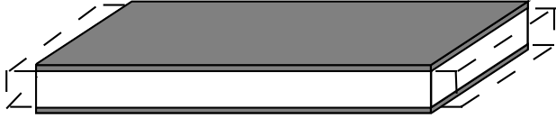
Figure 3. Lengthening effect ( d_{31}, d_{32} effect).
