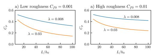
Figure 12: Sensitivity of farm-averaged power coefficient  $C_p$  to farm size ratio  $L/h_0$  for low ( $\lambda = 0.008$ ) and high ( $\lambda = 0.03$ ) array densities for a) low and b) high surface roughness values, for a fixed turbine resistance coefficient of  $C'_T = 1.33$ .
