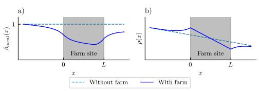
Figure 2: Example variations of a) local farm wind-speed reduction factor  $\beta_{local}(x)$  and b) pressure p(x) with streamwise location.
