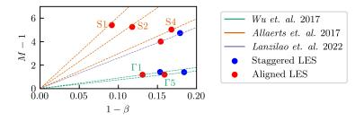
Figure 7: Predicted values of momentum availability factor (M) and farm wind-speed reduction factor ( $\beta$ ).  $\beta$  is calculated using equation 4.4 and M using equation 3.25 for the flow conditions and farm configuration used in the LES. Note that the lines are calculated using equation A 5.
