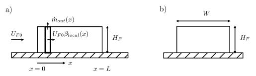
Figure 1: Control volume analysis for net momentum advection calculation a) side view and b) front view.
