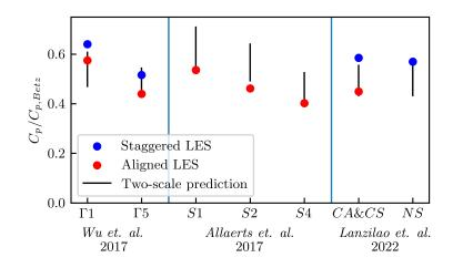
Figure 6: Comparison of farm-average performance predicted by the two-scale model and results from LES. The upper end of each black line corresponds to the upper limit of farm performance predicted by the two-scale model (i.e., without 'turbine-scale loss') whereas the lower end corresponds to the lower limit predicted assuming that the turbine-wake interaction causes a 20% reduction of  $C_T^*$ .
