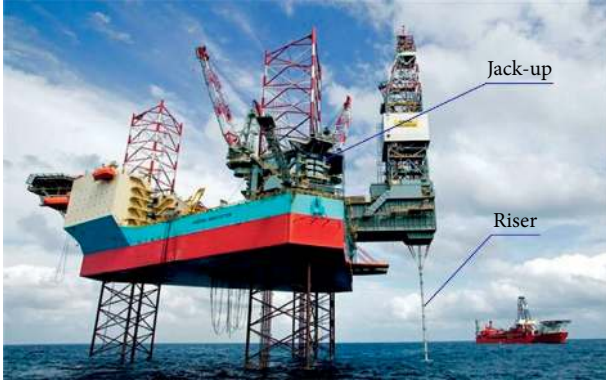
FIGURE 1: The working conditions of the jack-up platform with subsea BOP.
