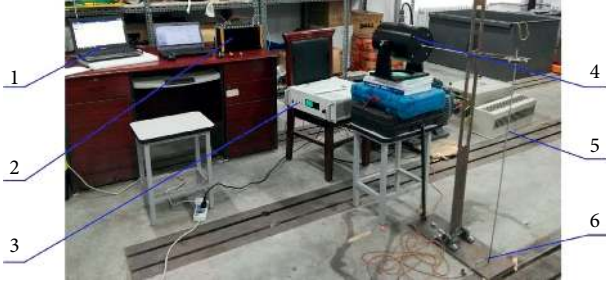
FIGURE 3: Diagram of the experiment system. 1, computer; 2, data analyzer; 3, power amplifier; 4, vibration exciter; 5, beam; 6, strain gauge.
