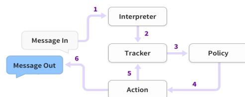
Fig. 1. Rasa architecture flow chart
