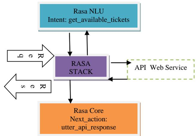
Fig. 5. API communication procedure
