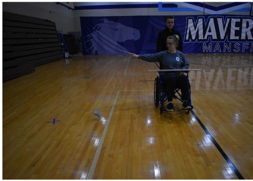
Fig. 7 The apparatus and setup for Experiment 3 is shown here. The participant sits in wheelchair and slides bean bag off of the wooden board as she is moving in the direction of the viewer of the photo at \sim 1.45 m/s
