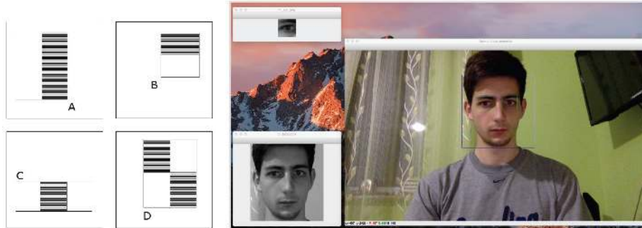
Fig. 3. Types of attributes used in the Viola-Jones algorithm Fig. 4. Face and Eye Recognition
