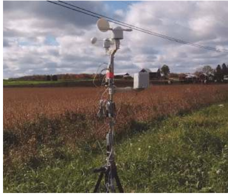
FIGURE 14: Weather sensing IoT system as utilized in a farm.
