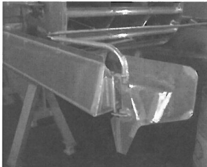
Figure 2: Hull extensions and rudder modifications
