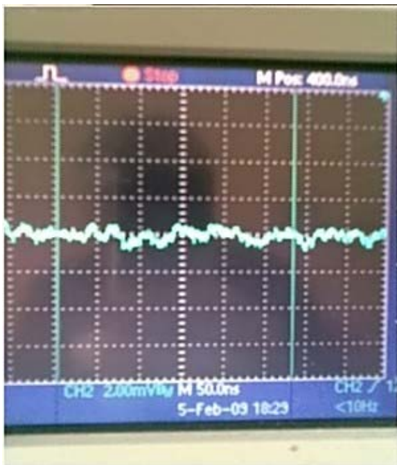
Fig. 15. SMPS +8V output after common mode filter (scale 2mV)
