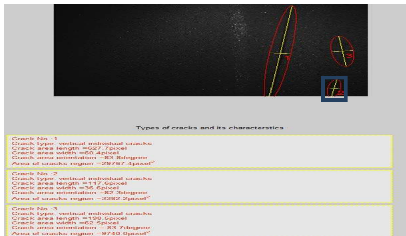
Figure B.11: An example of a false detection (second type of error) for case study (4).
