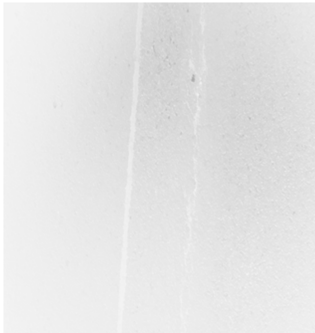
Figure 3.5: LEHMANN + PARTNER GmbH dataset, the resultant image after applying the dilate process; (inverted illustration).
