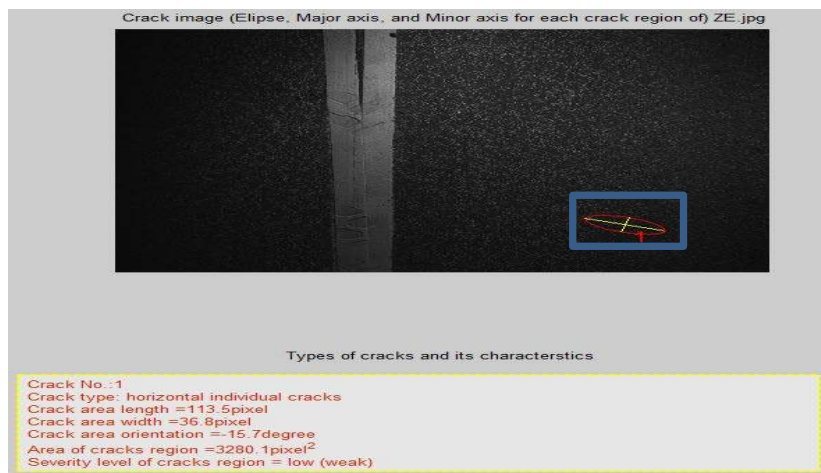
Figure B.10: A sample of a false detection (second type of error) for case study (3).
