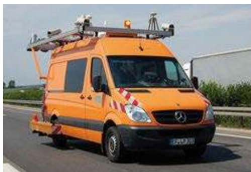
Figure 6.1: S.T.I.E.R. mobile mapping system (LEHMANN+PARTNER 2014).
