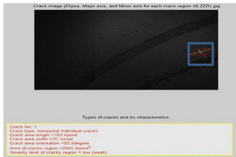
Figure B.9: A sample of false detection (second type of error) in case study (2).
