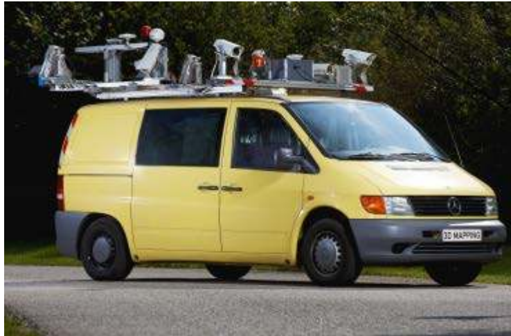
Figure 6.2: MoSES mobile mapping system (3D-MAPPING 2014).
