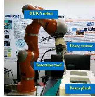
Figure 3: The experimental setup for the insertion task.
