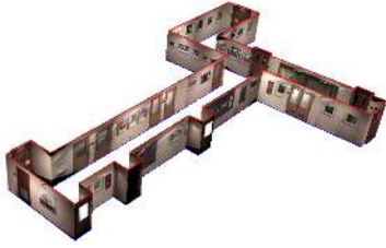
Fig. 11: Shown here is the 3D map reconstructed from the 333 pairs of training images used in the evaluation of the locale signature based approach to robot self localization.
