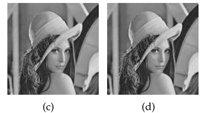
Fig. 15: The effect of different lengths of the stochastic bit streams on the gamma correction application. The lengths of the stochastic bit streams are (a) 128; (b) 256; (c) 512; (d) 1024.
