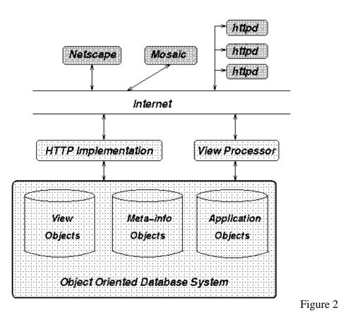
The system architecture is the key to supporting dynamically customizable views on the web. Our architecture is shown in Figure 2. It consists of three major components:
