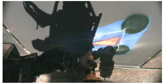
Figure 15: Top left: head camera view of poker used to press drill's power button. Top right: visualization of the nominal plan to reach all drill target points in the triangle. Bottom right: head camera view provides situational awareness to operator as robot executes drilling plan. Bottom left: Robot avatar and RGB point cloud visualization with affordance models of the drill and triangle target.
