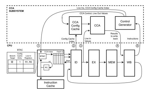
Figure 2: Transparent instruction set customization architectural framework
