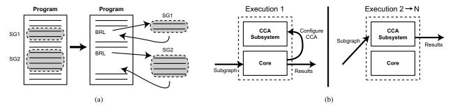
Figure 1: A high-level overview of the executing with a CCA: (a) subgraph identification and relocation and (b) setting up the CCA subsystem on the first invocation of a subgraph for future uses
