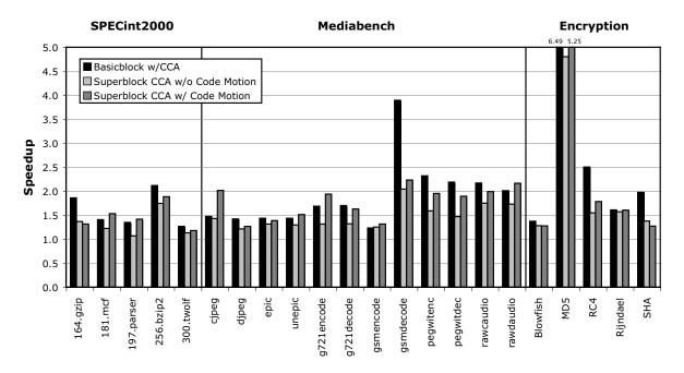
Figure 8: Speedup of basic block and superblock code when executing with a general purpose CCA
