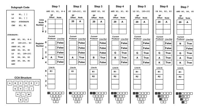
Figure 4: Example mapping subgraph onto a CCA
