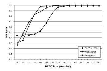
Figure 7: BTAC hit rate with various entry sizes
