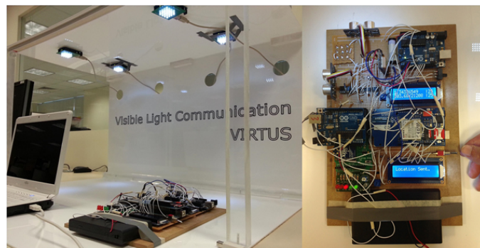
Fig. 1. Project setup and prototype of the 12V positioning receiver.
