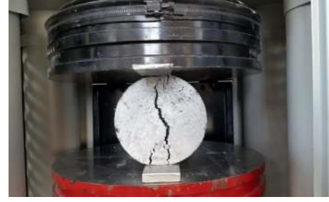
FIGURE 1: Split-tensile strength test.
