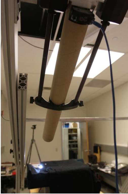
Figure 3-7. Tube covering the illuminance meter
