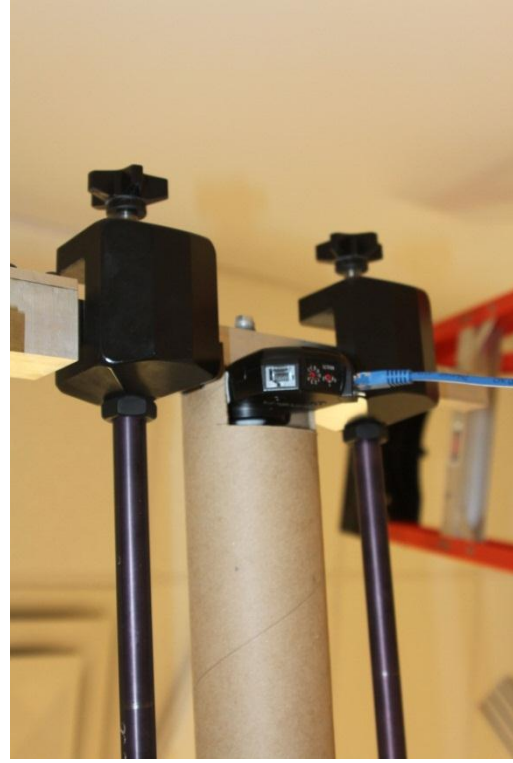
Figure 3-7. Tube covering the illuminance meter
