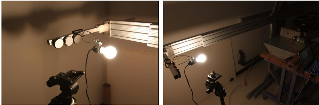
Figure F1. Experimental setting for making HDRI of the incandescent light source
