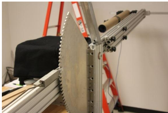
Figure 3-11. Changing gear in 2.5 degree increments
