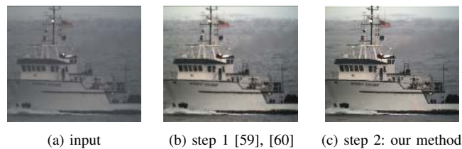
Fig. 12. Hot-air turbulence removal for the sequence “Acoustic Explorer” - using the proposed method to reduce the effect of hot-air turbulence. (a) A frame of the original video sequence. (b) Step 1: Apply gray level grouping [59], [60] to the input. (c) Step 2: Apply the proposed method to the results of Step 1.
