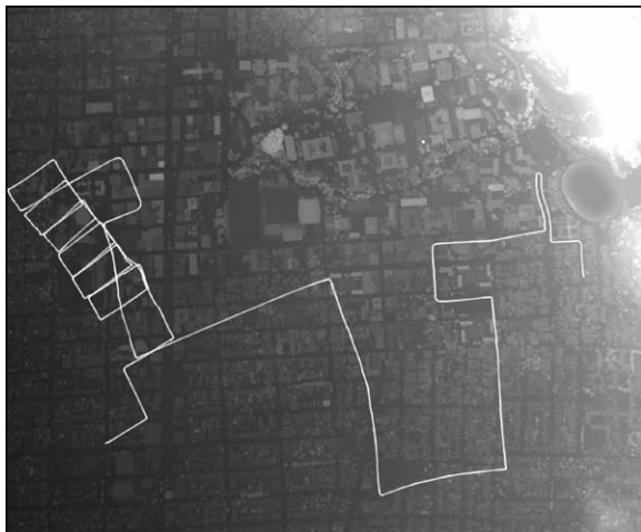
Figure 12. Initial path computed by concatenating relative pose estimates obtained in the scan-to-scan matching process, superimposed on top of the DSM.
