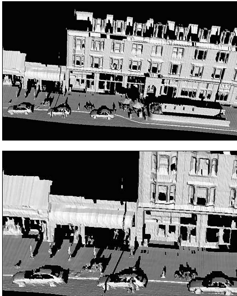
Figure 21. Surface mesh by triangulating the point cloud.
