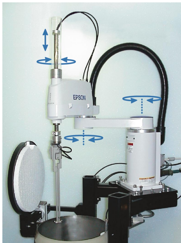
Figure 1 The Epson pick-and-place robot fitted with a pneumatic gripper actuator is shown. The four robot degrees of freedom are indicated by the arrows.
