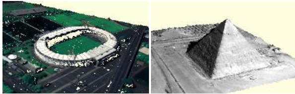
Figure 1: 3D point clouds automatically generated from Pléiades stereo datasets, without any manual intervention, with the s2p stereo pipeline. Its implementation can be tested online through a web browser.
