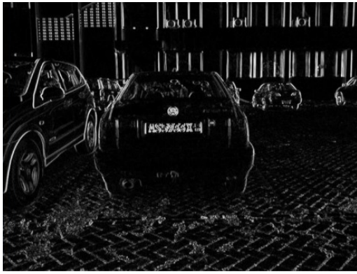
Fig. 7. Horizontal Sobel-Feldman convolution applied to image to determine horizontal edges of the plate.
