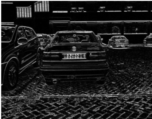
Fig. 8. Vertical Sobel-Feldman convolution applied to image to determine vertical edges of the plate.
