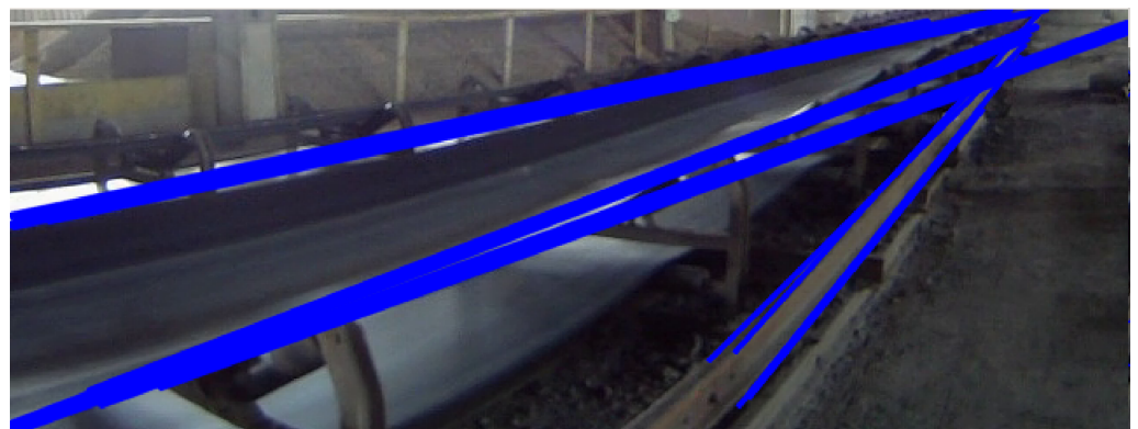
Figure 7. Exemplary effect of general line detection (Hough transform).
