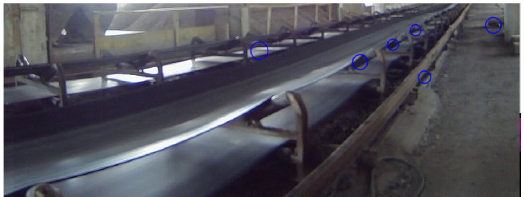
Figure 9. Example of incorrect idler blob detection.
