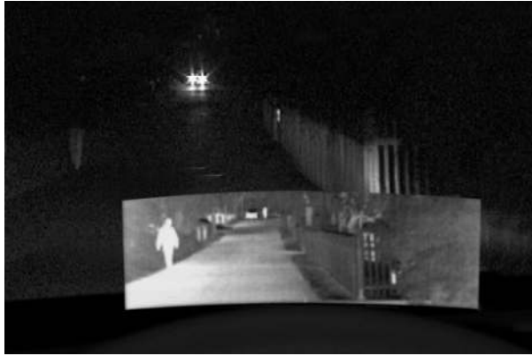
Figure 2.2: The night vision system of the Volvo Safety Concept Car. Photo: Volvo Car Corporation.
