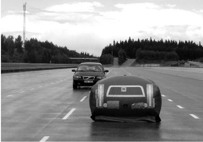
Figure 6.4: The test track and the inflatable dummy vehicle that was used in the ELA development.
