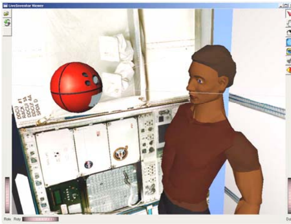
Figure 5 - 3D simulator screenshot of PSA in ISS with crewmember
