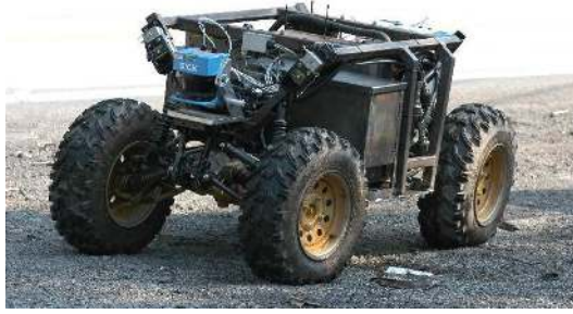
Figure 1: The Groundhog robot is a 1,500 pound custom-built vehicle equipped with onboard computing, laser range sensing, gas and sinkage sensors, and video recording equipment. Its purpose is to explore and map abandoned mines.
