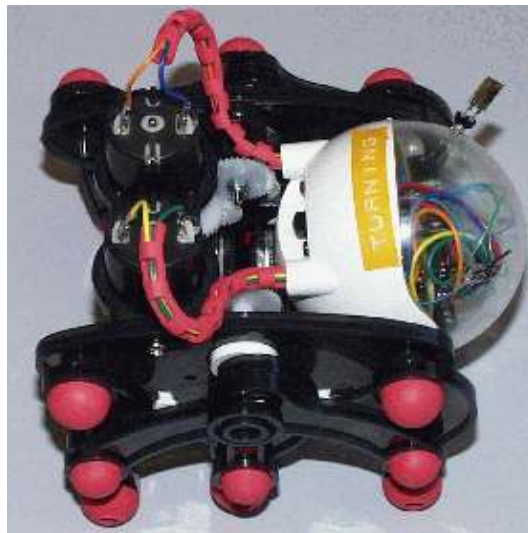
Figure 5: This robot, built from a toy kit produced by the Elekit company, contains only two sensors oriented at a 90^\circ from each other, with their mid-angle located along the robot's apparent line of motion. The robot is powered by two DC motors, each controlling one set of 'legs', and has a simple combinatorial logic controlling these motors.
