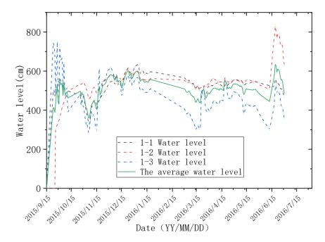
Figure 4. Variation in water level at different points on the same line of a rare earth slope with time.
