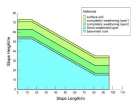
**Figure 9.** Slope model (with a slope height of 38 m and a slope angle of  $30^{\circ}$ ).
