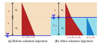
Figure 1. Slope models before and after solution injection.
