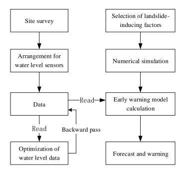
**Figure 2.** Operation flow chart of landslide warning system on the basis of the online monitoring of water level.
