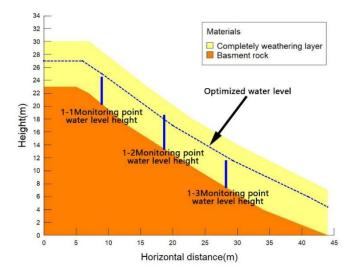
Figure 5. Schematic diagram of water level optimization.
