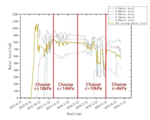
**Figure 11.** Principles of landslide early warning model at different leaching stages (c refers to cohesion in the figure).
