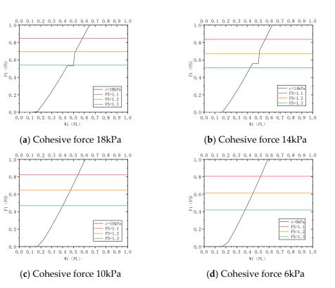
**Figure 10.** Landslide early warning model for ion-adsorption rare earth with a slope of  $\alpha$  30°.
