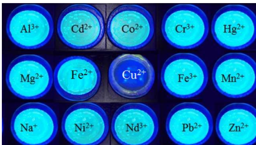
Fig. 15. Response of membrane sensors toward different metal ions. Distinct behaviour towards Cu 2+ is apparent from the figure.
