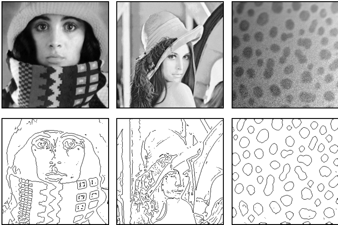
Figure 7: Presentation of the edge results achieved by applying our edge detector to "real world" images. In the shawl of bottom-left figure we notice a displacement of the detected edge position at sharp corners, caused by interference between these small spatial details and the size of the edge detector.
