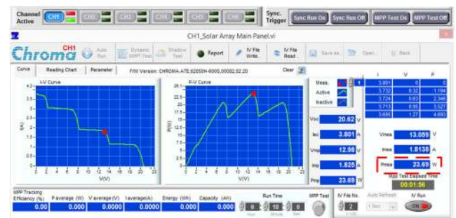
FIGURE 29. I-V and P-V curves under PSC for pattern 2.
