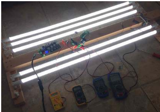
Fig. 12: Prototype of the series-remote driver zone light.
