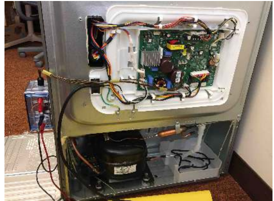
Fig. 8: Prototype for the DC input modification of a refrigerator. The blue box on the left side allows for a 340 V DC input to the inverter board’s DC capacitor bus. The compressor is the BMA069LAMV model.
