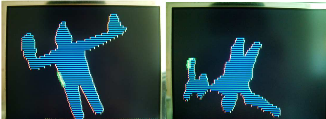
Fig. 7. The extracted contours of the segmented objects. The left-side contour points are marked in red whereas the right-side are in green. The highlighted bold green points move along the contour sequentially; we show these to help the reader visualize how the points are ordered.
