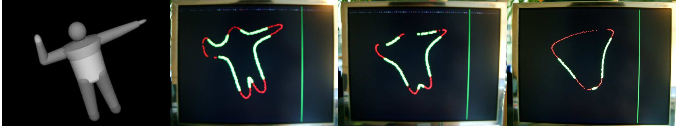
Fig. 8. The curvature zero-crossings on smoothed contours: The leftmost figure is the image of a 3D synthetic human model. Starting with the second left, the bold green contour segments indicate concave curvature and the thin red contour segments the convex curvature. From the left: \sigma=8, 40, 120 .
