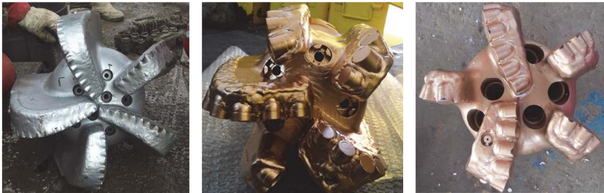
FIGURE 2: Three types of PDC drilling bits.
