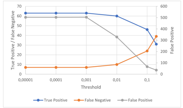
FIGURE 8. Number of false positive, false negative and true positive detections for the Kaggle dataset as a function of the detection threshold.
