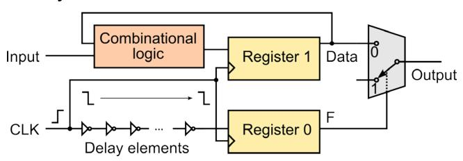
Delay elements could be used for enable signal generation in Li's countermeasure
