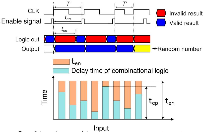
$\blacksquare$  Condition that enables countermeasure:  $t_{en} > t_{cp}$
