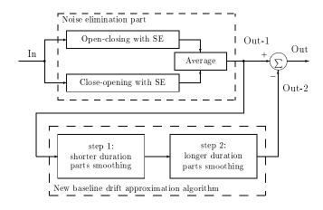
Figure 1: Simplified block diagram of ECG preprocessing (method 2).
