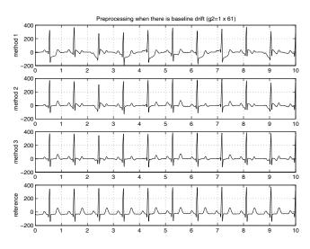
Figure 4: Baseline drift correction with three methods.
