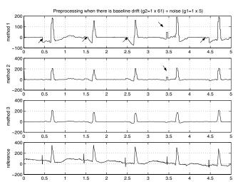
Figure 8: The preprocessing with three methods for the baseline wander correction at first and then, high frequency noise removal.
