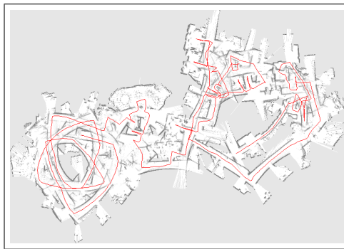
Fig. 11. Map created with the standard Rao-Blackwellized particle filtering technique in real-time using 100 samples and based on the raw odometry data.
