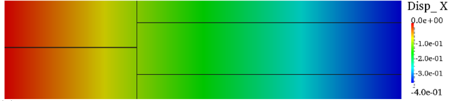
(a) Displacement contours in the x-direction at the maximum load for frictionless sliding along \Gamma .
