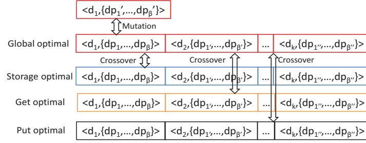
Figure 5.3: GA-based data allocation enhancement.
