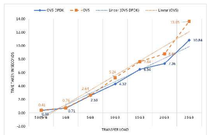
FIGURE 11. Time interval comparison between OVS and OVS-DPDK with varying load transfer
