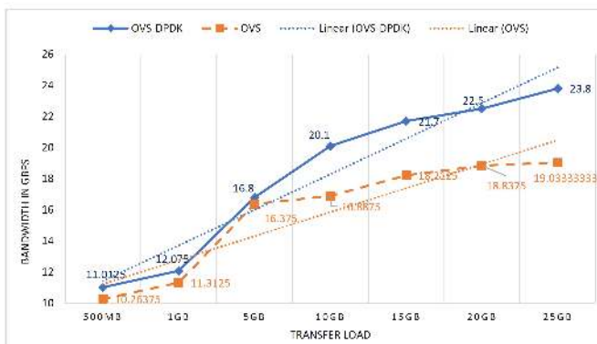
FIGURE 10. Performance comparison between OVS and OVS-DPDK with varying loads
